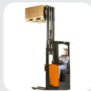
1. Lifting heights up to 6,5 m. Rocla designed integral mast in 2000 kg model enables automatic lift stop at wished lifting height.
