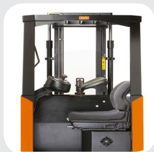
2. New comfortable seat and ergonomic driving position. The b2 control panel has a completely new digital display and control buttons in the middle.
